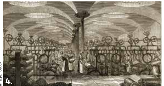
4. Adequate light for machinery and workers necessitated larger building volumes during the Industrial Revolution.
